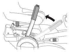
2 For Rider 11 C Pull back the throttle and move the gear shift lever to the neutral position "N", without pressing in the reversing lock button. Turn the ignition key to the "STOP".
